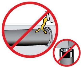
Only fill pump to recommended level, and fill only when the connected cylinder is fully retracted.
