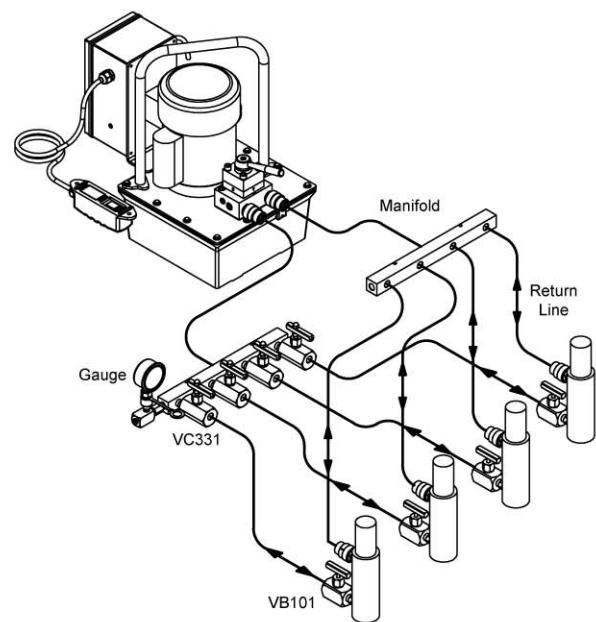
Many different system arrangements can be achieved by using a remote mounted directional valve. Remote valves are ideal when system control is desired away from the pump. Hydraulic connections are quick and convenient when you use inline manifolds to control up to 4 double-acting cylinders.
