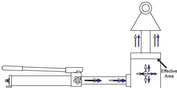
The basic hydraulic system consists of a single acting cylinder. The pump can be powered by an electric motor, air power and also mechanic driven by hand or foot pumps.
