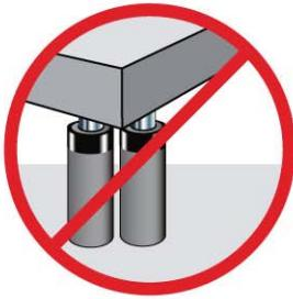
For multiple rams lift, you must be able to determine the location and number of lifting points that will allow the load to be evenly distributed to all the rams. This is called load balance. Size, center of gravity, and load geometry must be considered in order to correctly determine load balance.
