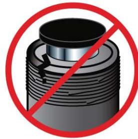
Check each component before you set up your hydraulic system. Do not use damaged or worn components. Turn them in for repair or replacement.
