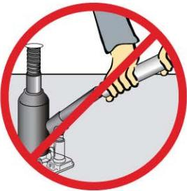
Do not use extensions or cheater bars on hydraulic jacks or hand pumps to raise a load.
