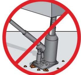
Every jack or ram, whether used individually or in a system, should be completely supported on a solid, firm, non-sliding foundation capable of supporting the load.
