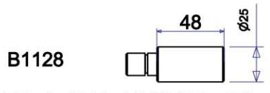
Extension Rod for 4, 6, 8 & 12 Tons Pullers
