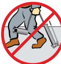
Dragging or carrying rams or pumps by a connected hose can damage the couplers and hoses. Using damaged couplers and hoses can be dangerous.
