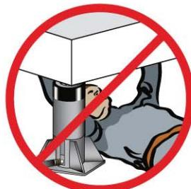
Hydraulic rams are not meant to be used as permanent supports, but are designed to lift and lower. If you need to hold the load for any length of time, cribbing or Powerram locknut cylinders should be used.
