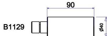
B1129 Extension Rod for 20 & 30 Tons Pullers
