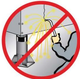
Weld splatter will damage plunger rods and hoses. Hydraulic fluid can ignite if vaporized or exposed to high temperatures.
